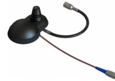
Roof mounted universal antenna base with built-in active GNSS antenna. The base accepts mobile antenna whips with external M5 threaded stud. M5/M6-adaptor for optionally mounting of antenna whips with internal M6 thread is supplied
