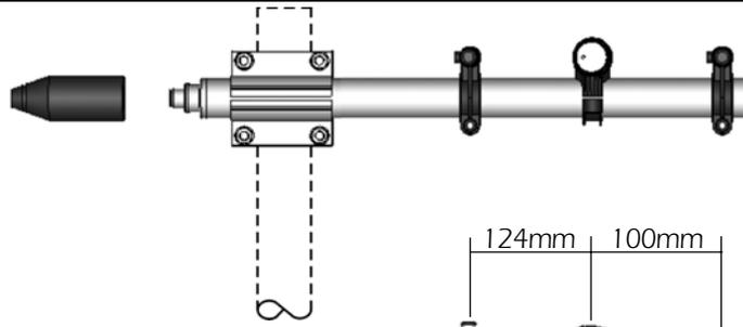
**Correct mounting for vertical polarization**
