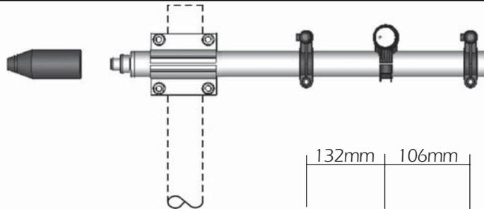
**Correct mounting for vertical polarization**
